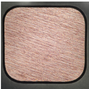
近似方形铜线实物剖面写真 Square-like Enamelled Wire Section View
